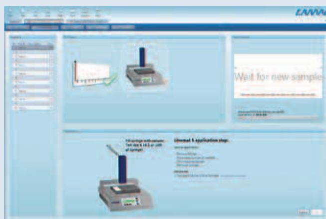
For operation under visionCATS as well as under winCATS, the display shows the status of the instrument and the progress of the current application.
