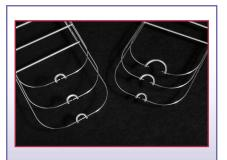
Patented ARCH Probes Designed for Dissolution Testing Eliminate bubble formation and particulate entrapment that plague other fiber systems
